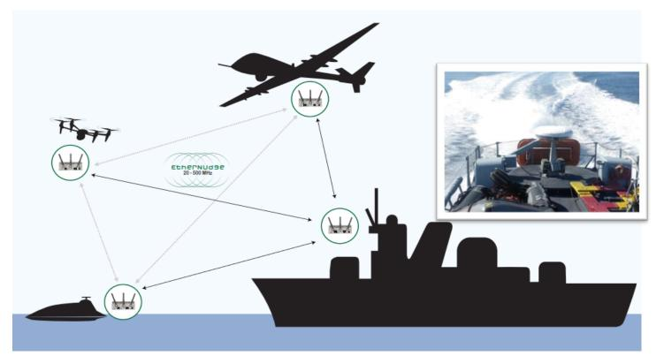
The "Super-Cell" is a LAN environment, in which the ethernet-line is being extended through the air, supporting all IP/LAN based applications without delay and with exceptional performance even without line-of-site (LOS) on rough seas.
